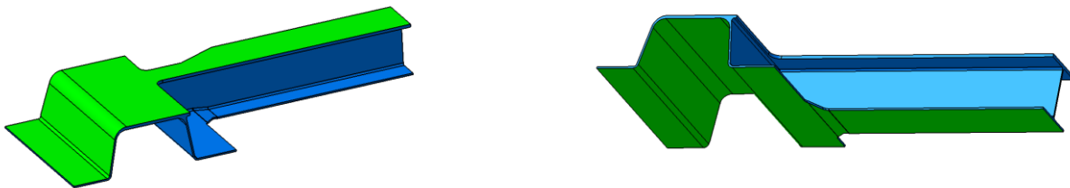
Figure 14: Transverse Stiffener: surfaces with shape/flatness requirement.
